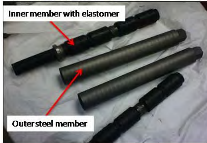
Figure 4. Picture of bit isolator design, two units disassembled.
