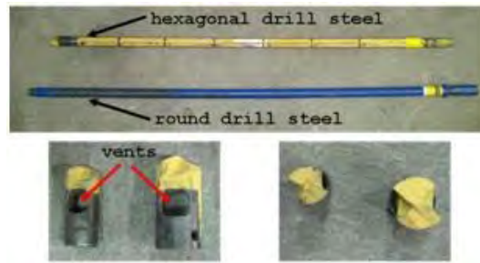
Figure 1. Hexagonal and round drill steels for a 1 3/8" (35-mm) diameter drill bit (upper) and two examples of drill bits (lower) – 1" and 1 3/8" (25 mm and 35 mm).
