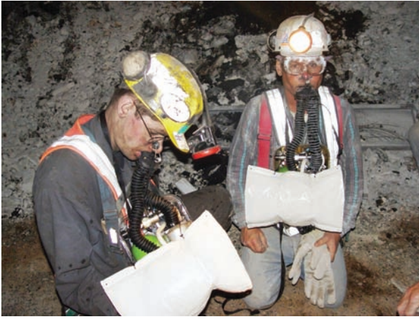
FIGURE 1. Miners wearing compressed oxygen SCSRs during a simulated escape
