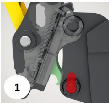
1 Misconnection – Operator thinks the bucket is correctly attached.
