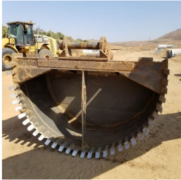
The bucket that disconnected from the coupler in Case Study #1. Photo: CA FACE program
