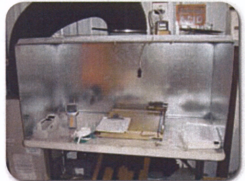
Enclosing hood with HEPA exhaust constructed to control possible emission of nylon nanofibers during destructive testing.
