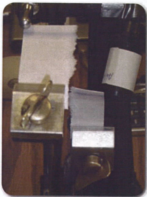
Air sampling filter in close proximity during tear-testing of nanofiber coated cellulose.
