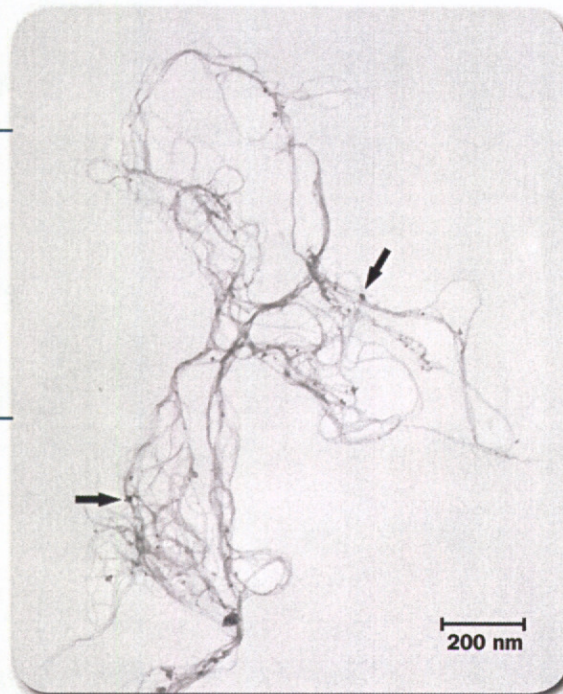
SWCNTs produced by the high-pressure decomposition of carbon monoxide (HiPCO) method. Arrows note iron contamination of the unpurified SWCNT.
