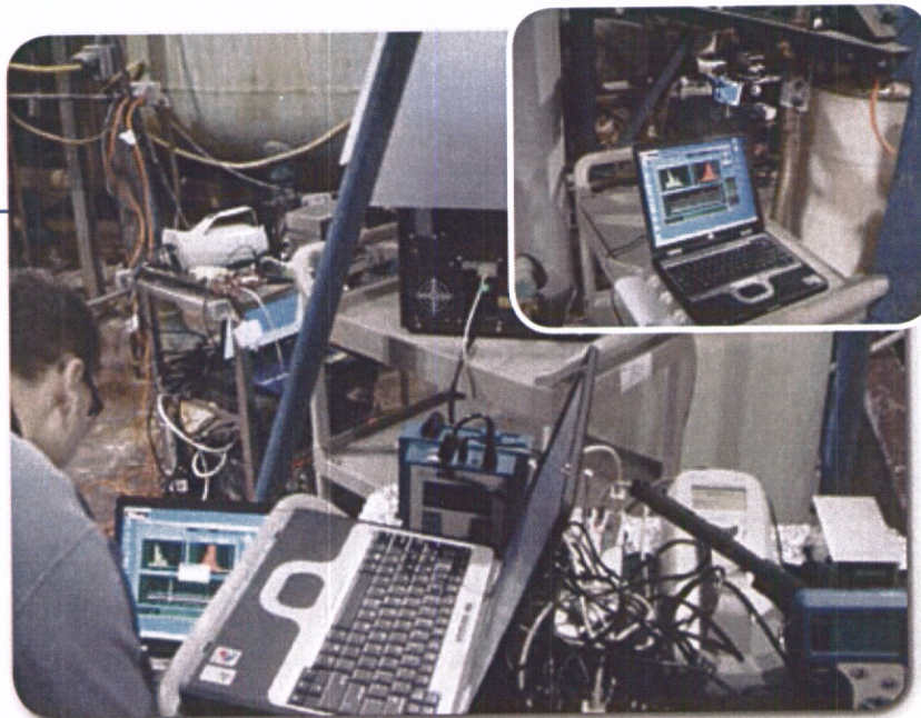
Comprehensive aerosols measurements conducted at different production processes within a primary nanoscale metal oxide production facility. A number of aerosol sampling methods and instruments are used simultaneously to better understand particle characteristics.
