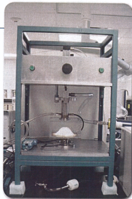
A flat plate test system for measuring respirator filter penetration of 3 to 20 nm silver particles
