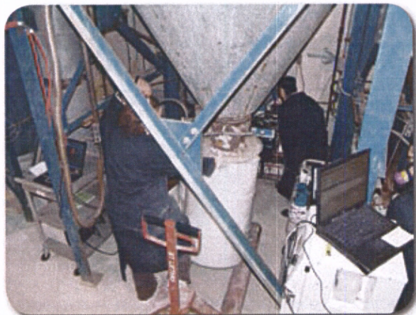
Sampling for airborne nanoparticles during a drum changing operation in a commercial nanomaterial production facility.
