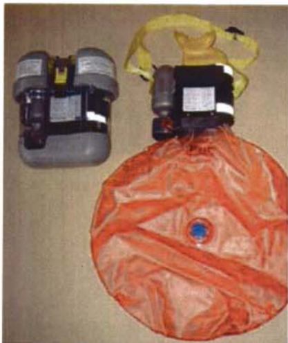
Figure 7. Partially Uncased and Uncased Ocenco M-20 Self-rescuer
