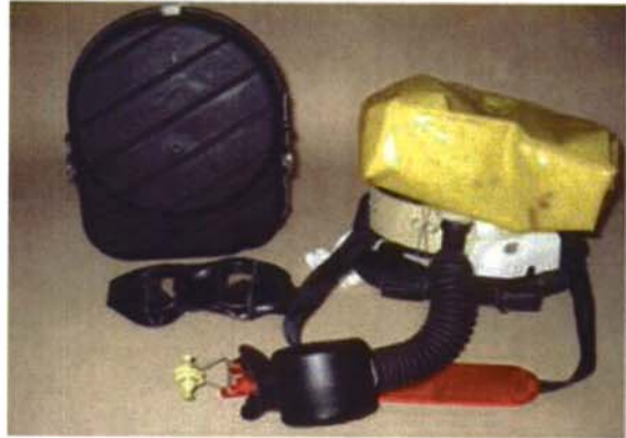
Figure 4. Cased and Uncased Draeger OXY K-Plus Self-rescuer
